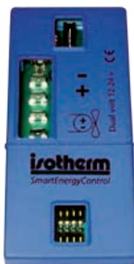
The Smart Energy Control (SEC) is a sophisticated processor-based control device, that achieves significant power consumption by continuously scanning a set of key environmental factors, to operate the compressors at their best performance/battery drain ratio. Via the storage function in food and drinks can achieve up to 50% savings Vs. conventional control systems, representing the best answers for users hunting for the lowest power consumption.
