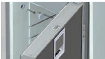
The new installation system allows an easy fixing of the cabinet directly from the interior of the fridge. The external flange is no longer necessary for the installation. An innovative internal bushing structure prevents the crushing of the insulated side wall.
