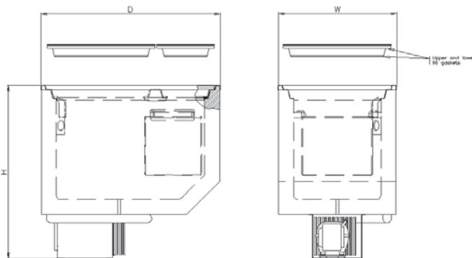
The CRUISE 40 Cubic can also be installed as a built-in top opening cooler box.
